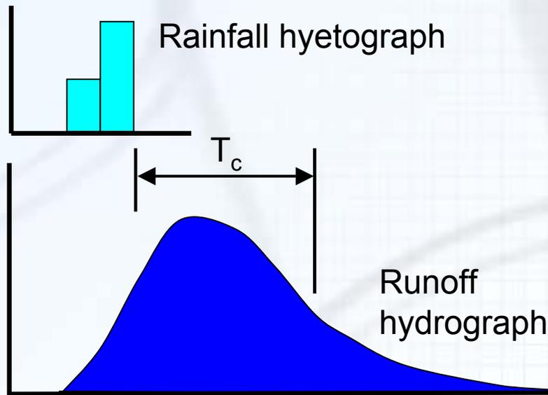
$T_c$  is a function of area, slope, surface roughness and rainfall intensity
