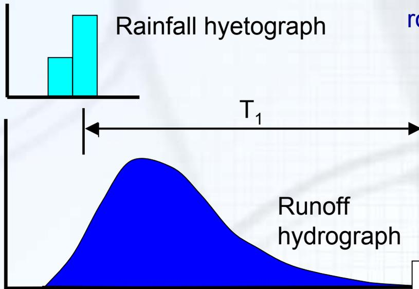
$T_1$  is a function of area, slope, surface roughness and rainfall intensity
